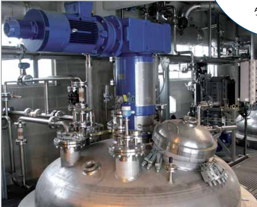
Top entry reactor used in the pharmaceutical industry
