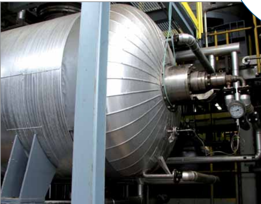
Horizontal dryer used in the chemical and pharmaceutical industries
