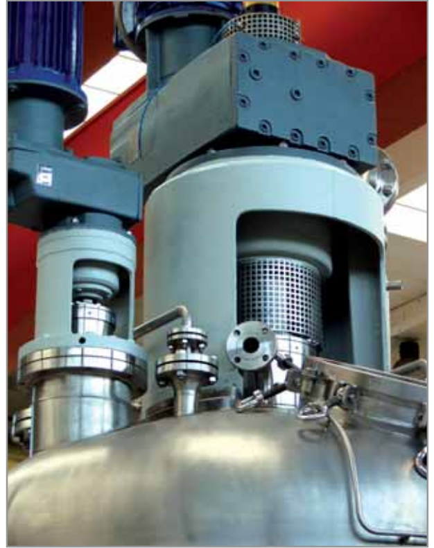
Double cartridge seal on a top-entry agitator
