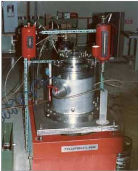
Dual reactor seal designed and tested for Pressindustria in 1985. They were installed in a large rubber production plant in Russia
