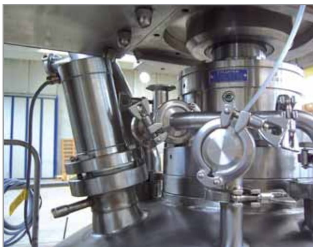
Dual mechanical seal for dry running in sterile conditions
